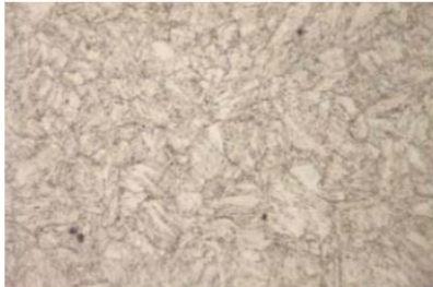
Fig. 1. Non-equilibrium microstructure of a S960QL (WELDOX 960 E by SSAB), N=1000x, 2% HNO 3 [3]
